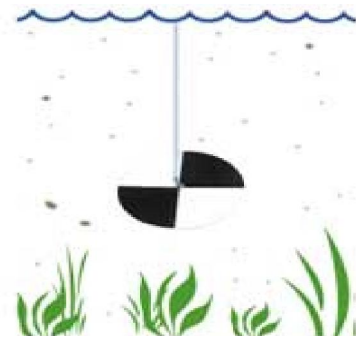
A clear lake with small algal populations results in deep Secchi disk readings and low levels of chlorophyll-a and TP.
